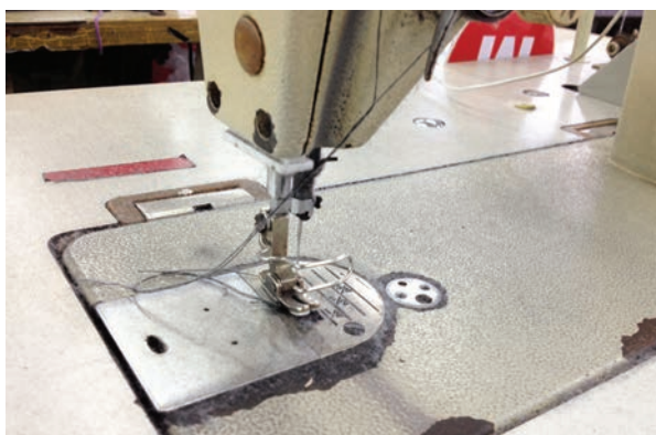
Needle guards installed
