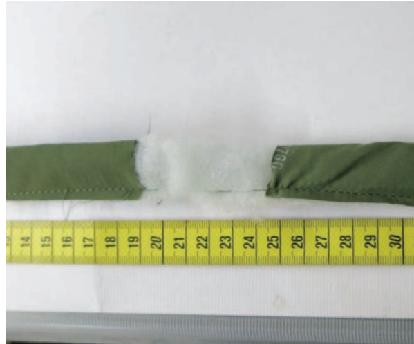
Inner lining wastage of 5 cm
