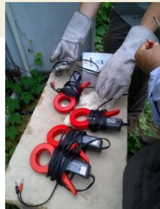
Electricity data logger and its clamp current transformers
